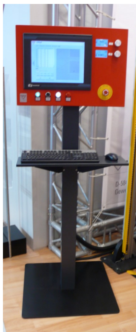
Operating terminal with industrial panel PC and software i3stud (with DXF data converter)
