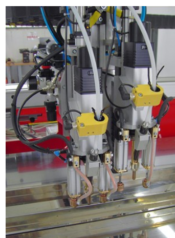
Grounding by pneumatic cylinders mounted on welding head
